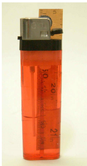
Figure 2. The half-filled disposable lighter used in the second part of the experiment demonstrating spontaneous distillation.
